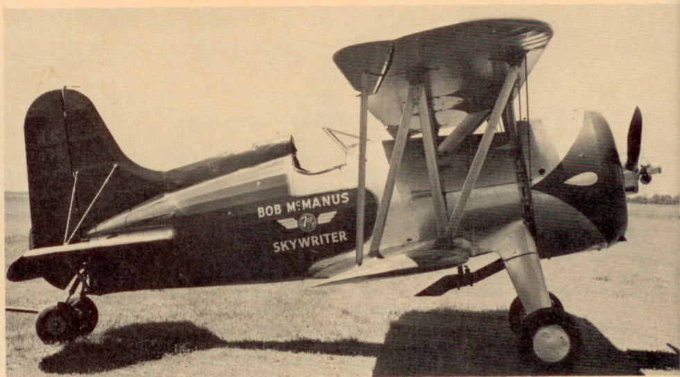
Postwar modification of the Boeing 100A added a constant-speed propeller and a single-strut landing gear. The high tail had been added in the 1930s, before Hughes sold the plane to Art Goebel.
